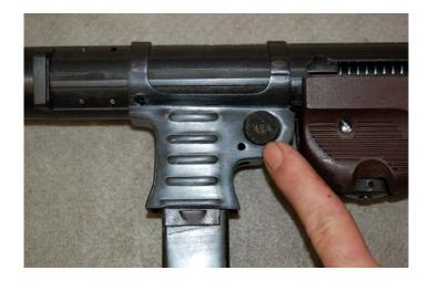
Depress the button with your finger and pull the magazine down and out of the gun.
