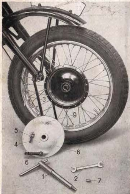
Fig. 1 Disassembly of the front wheel.
